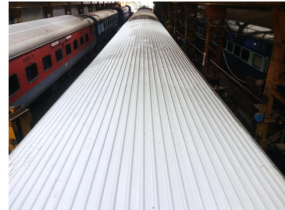
APPLICATION OF FIRST COAT OF THERMACOOL 0.3M FR
